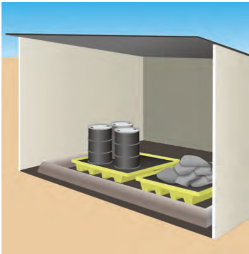
Figure 15. Illustration showing construction materials with secondary containment and overhead cover to prevent stormwater contamination.
